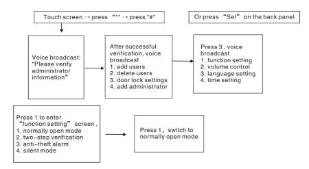
Note: After the normally open mode is turned on, each time when unlocking, the lock will enter the normally open state, press "#" to lock.
