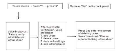
Note: To delete the user, fingerprint/card user must verify the unlocking information.
